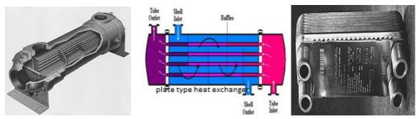
In shell and tube type heat exchangers the cooling fluid flows in the bunch of tubes placed in side the shell while the fluid to be cooled flows, in a reverse direction, in the shell, in the leftover gaps between the tubes.
