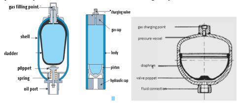
Accumulator is used (a) for smooth functioning of HS without pressure and flow fluctuations (b) as an emergency power source for essential operations in case of power failure. (c) for holding pressure for long times in a circuit (d) a big pump can be replaced by a small pump (cost & energy saving) and many other purposes.
