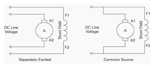
In a shunt motor the field is connected in parallel (shunt) with the armature windings. The shunt-connected motor offers good speed regulation. The field winding can be separately excited or connected to the same source as the armature
