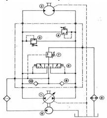
In the closed hydraulic the oil after rotating the hydro motor doesn't go to the tank back, instead it goes to the pump's suction line again. In this process the same oil is only circulating. To take care of the mixing of cool and fresh oil from the tank a booster pump is installed which is normally in tandem with the main pump. It mixes the oil from the tank to the circuit through a flushing valve.
