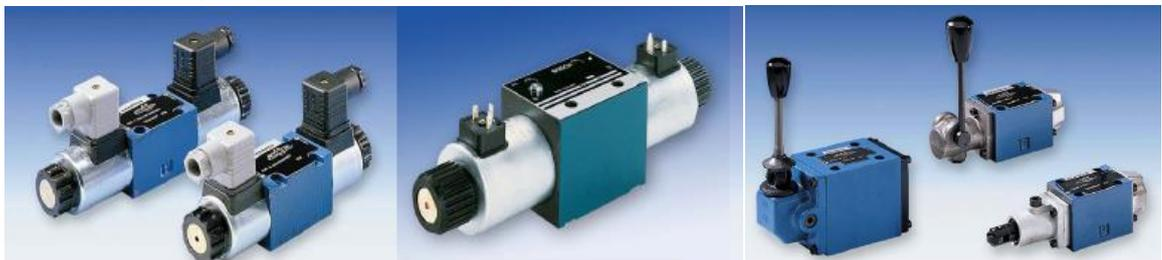
**FLOW CONTROL VALVES:** To control the speed of the actuator /load, the amount of oil flowing into the cylinder is controlled by means of these valves. Generally these are provided before the cylinder or in branch circuits where flow is to be controlled. Simple needle/globe valve can also be used as flow control valve in some cases.
