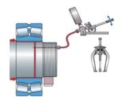
This method can't be used unless provided for in the design of mounting. Special oil injection tool is required. After mounting of bearings the axial float of the bearing should be as per OEM recommendation.
