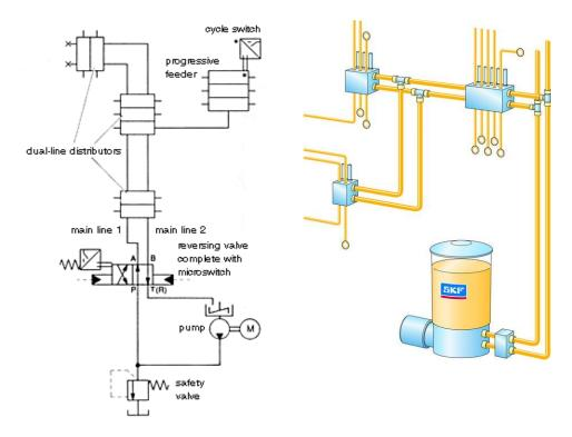
A typical dual line system flow diagram
