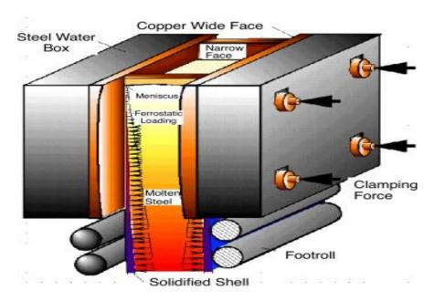
The mould is basically an open-ended box structure, containing a water-cooled inner lining fabricated from a high purity copper alloy. Mould water transfers heat from the solidifying shell. The working surface of the copper face is often plated with chromium or nickel to provide a harder working surface, and to avoid copper pickup on the surface of the cast strand.
