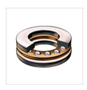
Ball thrust bearings like the one shown are mostly used for low-speed non precision applications. They cannot take much radial load and are usually found in low precision farm equipment. Thrust ball bearing designated as 5XXX.
