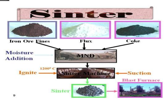
Sintering of fines by the under grate suction method consists of the mixing of fines
