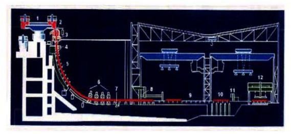
1:Ladle Turret, 2:Tundish/Tundish Car, 3:Mould, 4:First Zone (Secondary Cooling), 5:Strand Guide (plus Secondary Cooling), 6:Straightener Withdrawal Units, 7:Dummy Bar Disconnect Roll, 8:Torch Cut-Off Unit, 9:Dummy Bar Storage Area, 10:Cross Transfer Table, 11:Product Identification System, 12:Product Discharge System
