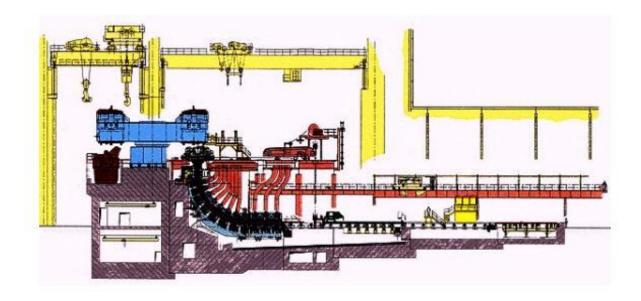
Figure 3 -Slab Caster Layout
