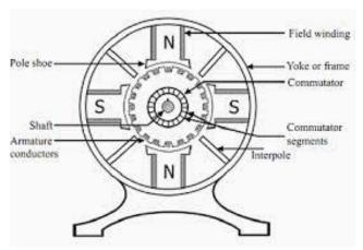
The outer frame of the motor is called yoke that serves two purposes.
