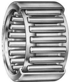
A variation of roller bearing design is called the needle bearing. The needle roller bearing uses cylindrical rollers like those above but with a very small diameter. This allows the bearing to fit into tight places such as gear boxes, cardan shafts that rotate at higher speeds & also has a more load carrying capacity.
