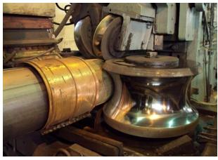
Hot rolled coils (from Hot Strip Mill of RSP or from out side sources like BSL) are the main input material for ERW Pipe Plant. This input material is cold formed to a tubular shape by gradual deformation and then welded by the combination of heat and pressure.
