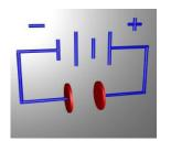
A parallel plate capacitor is shown in the adjoining figure, connected to a battery. The potential difference across the plates of the capacitor is equal to the battery voltage, thereby charging the capacitor. However due to the inherent nature of
