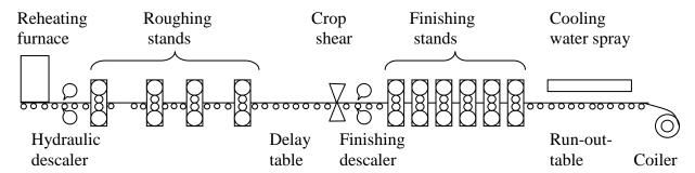
Process installations shown in the figure above and operations performed are briefly described below:
