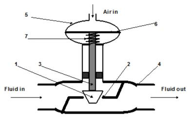
Fig.1 Air-to-close pneumatic actuator with valve
