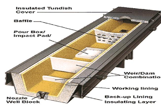
The shape of the tundish is typically rectangular, but delta and "T" shapes are also common. Nozzles are located along its bottom to distribute liquid steel to the moulds. The tundish also serves several other key functions:
