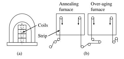
Figure: Schematics of (a) Batch Annealing and (b) Continuous Annealing
