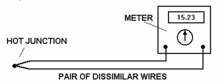
Most thermocouple metals produce a relationship between the two temperatures and the e.m.f as follows.
