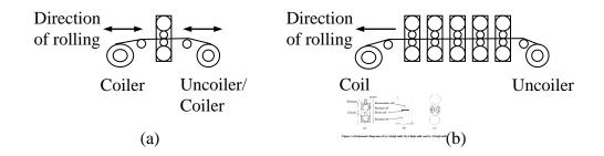
Schematic of (a) Reversing Mill and (b) Tandem Mill
