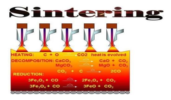
The gases used in ignition furnace are mainly coke oven gas or mixed gas. Mixedgas is combination of coke oven gas and blast furnace gas. Further the combustion is continued due to suction of air through the layers of the charge by means of Exhausters. Due to this, the process of combustion of fuel gradually moves downwards up to the grates.
