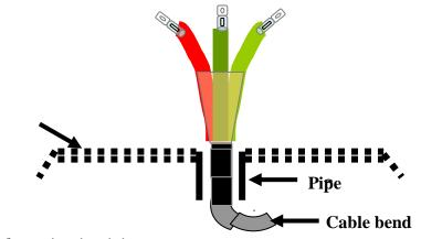
View of an end-termination joint
