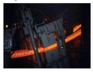
After straightening, the strand is transferred on roller tables to a cut off machine, which cuts the product into ordered lengths. Sectioning can be achieved either via torches or mechanical shears. Then, depending on the shape or grade, the cast section will either be placed in intermediate storage, hot-charged for finished rolling or sold as a semi-finished product.
