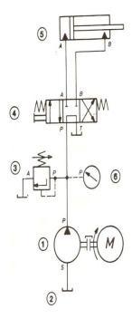
Generally pump is always followed by a Relief valve and then a NON RETURN VALVE (CHECK VALVE).
