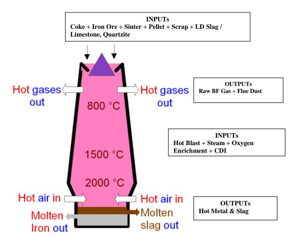
The entire furnace is lined with suitable refractory and in addition to refractory lining, there are water coolers, designed to enhance the life of the furnaces. In a blast furnace, fuel, Iron ore, sinter and flux (limestone) are continuously supplied through the top of the furnace, either through 'double bell system' or 'bell less system'. In the hearth, there is a tap hole of suitable dimension and length, for the purpose of tapping the hot metal.
