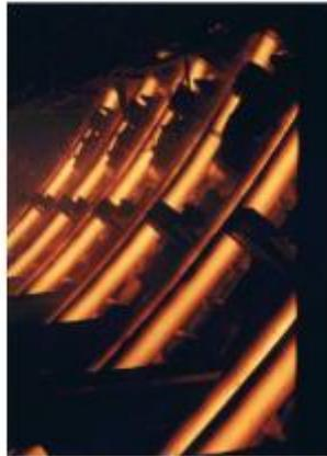
**Figure 8 - Straightener Withdrawal Units for Strand Unbending**
