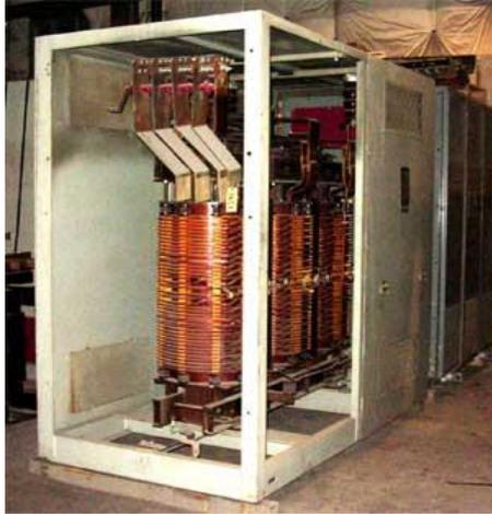
Distribution and thyristor transformers have all three insulating media. There are two types of dry-type transformers – cast-resin and vacuum pressure impregnated. However absence of an external coolant / insulating medium limits their capacity (up to 15 MVA).
