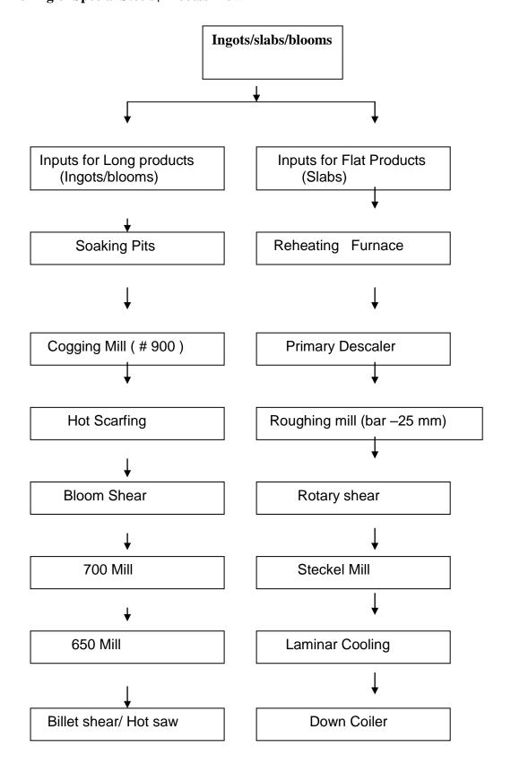
Special steels including Alloy and Stainless have both continuous cast and Ingot teeming products. Grades having high carbon and high alloy are hot transferred. All ingots and continuous cast slab or blooms are charged into soaking pit furnaces.
