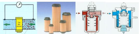
In a filter the hydraulic oil is allowed to pass through a porous medium (like clay, paper, wire mesh, synthetic fiber etc) so that the dust particles and other contaminants are retained and only clean oil goes ahead into the system.
