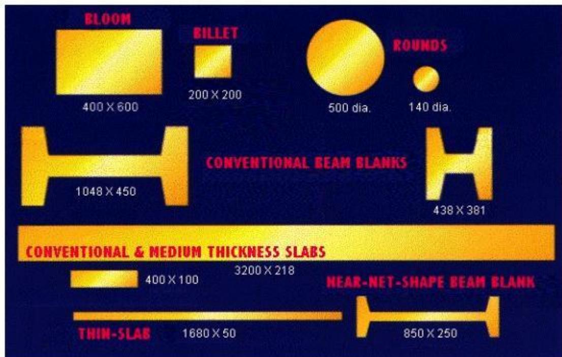
Figure 4 - Continuous Cast Shapes (sizes in millimeters)
