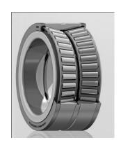
Tapered roller bearings are designed to support large radial and large thrust loads. These loads can take the form of constant loads or shock loads. Tapered roller bearings are used in many gear boxes, where they are usually mounted in pairs facing opposite directions. This gives them the ability to take thrust loads in both directions. Taper roller designated as 3XXX in metric size & in inch size 9XX/9XX.
