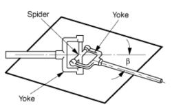
The angle between the two shafts is called the operating angle
