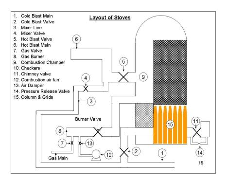
Hot Blast Stove and its Valve Arrangement
