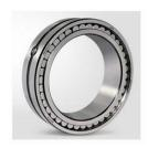
Cylindrical roller bearings generally are single row bearings with a cage. High-capacity bearings, double row bearings, multi-row bearings, single, double and multi-row full complement bearings (without a cage) and split bearings are other varieties. Bearings with a cage can accommodate heavy radial loads, rapid accelerations and high speeds. Full
