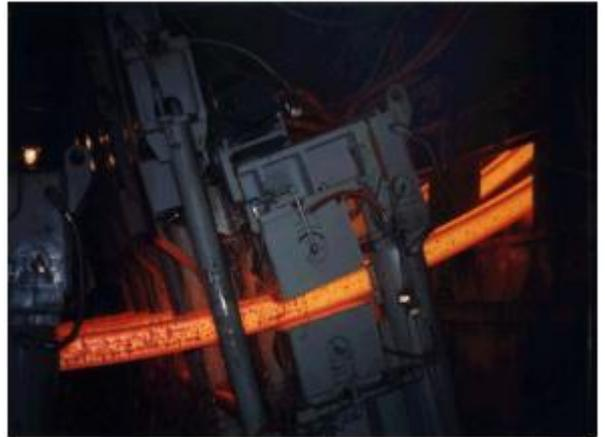
After straightening, the strand is transferred on roller tables to a cut off machine, which cuts the product into ordered lengths. Sectioning can be achieved either via torches or mechanical shears. Then, depending on the shape or grade, the cast section will either be placed in intermediate storage, hot-charged for finished rolling or sold as a semi-finished product.
