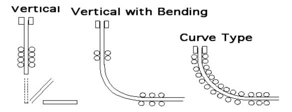
Steel from the electric or basic oxygen furnace is tapped into a ladle and taken to the continuous casting machine. The ladle is raised onto a turret that rotates the ladle into the casting position above the tundish. Referring to Figure 2, liquid steel flows out of the ladle
