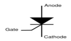
unidirectional conduction. The term **Thyristor is often** used in literature as a synonym of the SCR.
