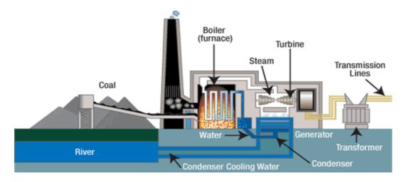
CPPs in SAIL are coal / gas-based thermal power plants. In thermal power stations, mechanical power is produced by a steam turbine, which transforms thermal energy, from combustion of a fuel (coal or by-product gases), into rotational energy. Pulverized coal is fed to the boiler, where its combustion takes place, thereby producing thermal energy that heats the water inside the boiler tubes. High pressure, high temperature steam then passes
