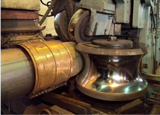
**Hot rolled coils** (from Hot Strip Mill of RSP or from out side sources like BSL) **are the main input material** for ERW Pipe Plant. This input material is cold formed to a tubular shape by gradual deformation and then welded by the combination of heat and pressure.
