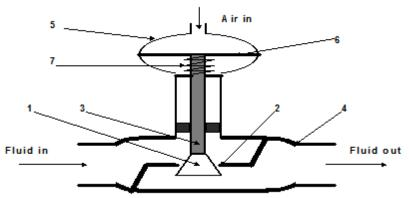
Fig.2 Air-to-open pneumatic actuator with valve
