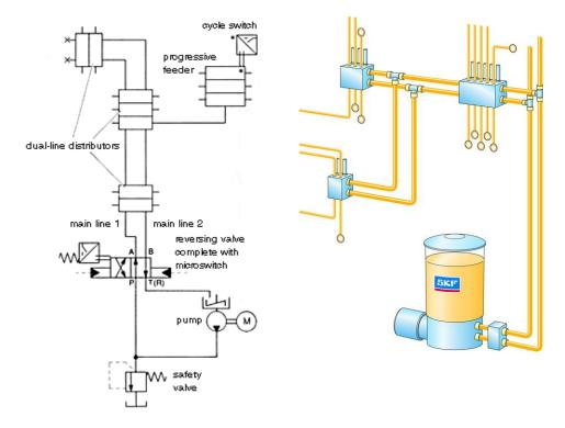
A typical dual line system flow diagram
