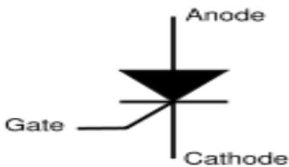
A thyristor usually has three electrodes: an anode, a cathode, and a gate (control electrode). When the anode is positive w.r.t. cathode (forward biased) and a pulse is applied to the gate, the SCR begins to conduct, and
