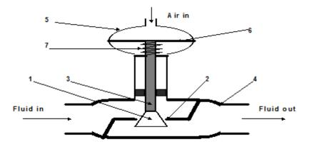
Fig.2 Air-to-open pneumatic actuator with valve
