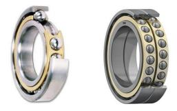
Ball bearing is a common bearing found in electric motor & centrifugal pump. These bearings are capable of taking both radial and axial loads and are usually found in applications where the load is light to medium and is constant in nature (ie not shock loading). Deep groove & angular contact type are two variety of ball bearing designated as 6XXX & 7XXX.
