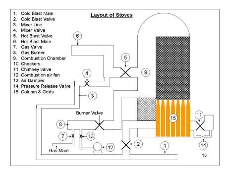
Hot Blast Stove and its Valve Arrangement
