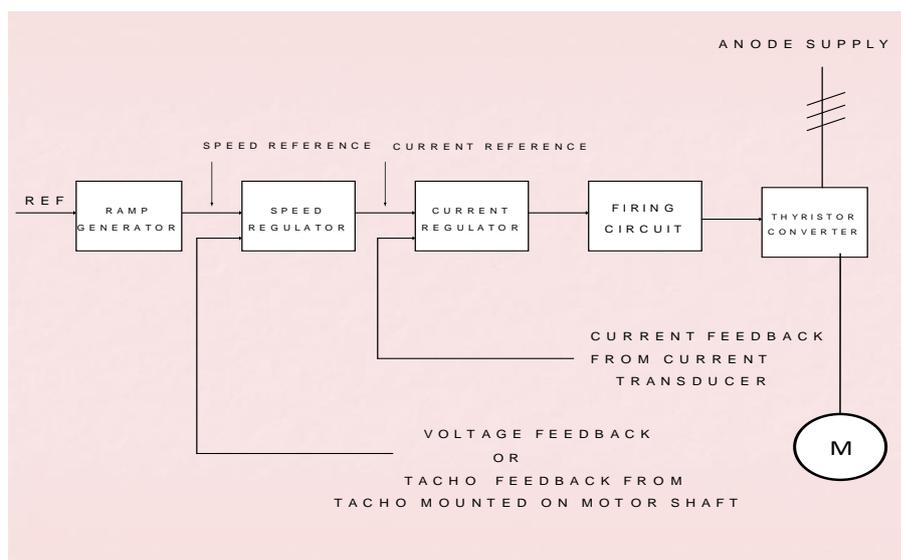
Fig.6 Diagram showing closed loop control of a typical dc motor (armature)
