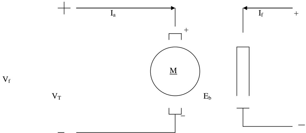
The figure above indicates typical configuration of a separately excited DC motor.
