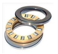
Roller thrust bearings like the one illustrated can support very large thrust loads. They are often found in gear sets like car transmissions between gear sprockets, and between the housing and the rotating shafts. The helical gears used in most transmissions have angled teeth, this can causes a high thrust load that must be supported by this type of bearing. Roller thrust bearing designated as 8XXX
