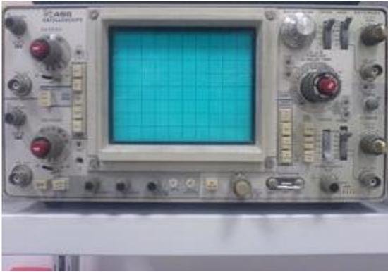
An **oscilloscope** (sometimes abbreviated **CRO**, for cathode-ray oscilloscope, or commonly just **scope** or **O-scope**) is a type of electronic test equipment that allows signal voltages to be viewed, usually as a two-dimensional graph of one or more electrical signals (on the vertical axis) plotted as a function of time or of some other voltage (on the horizontal axis). A typical CRO has a small screen on its front panel on which the graphs are displayed when the inputs
