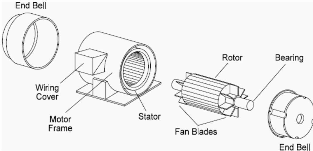
AC Motor uses electrical energy in AC form to convert it into mechanical energy
