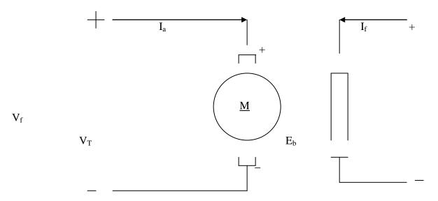
The figure above indicates typical configuration of a separately excited DC motor.
