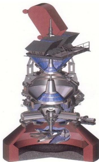
Fig-3 Rotary Charging Unit (RCU)
