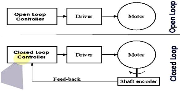
Closed loop VS Open loop
