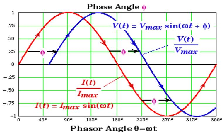
The angle by which the sine curve of the voltage in a circuit leads or lags the sine curve of the current in that circuit is called the phase angle  $\phi$ . If  $\phi$  is positive the voltage leads the current.
