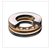
Ball thrust bearings like the one shown are mostly used for low-speed non precision applications. They cannot take much radial load and are usually found in low precision farm equipment. Thrust ball bearing designated as 5XXX.
