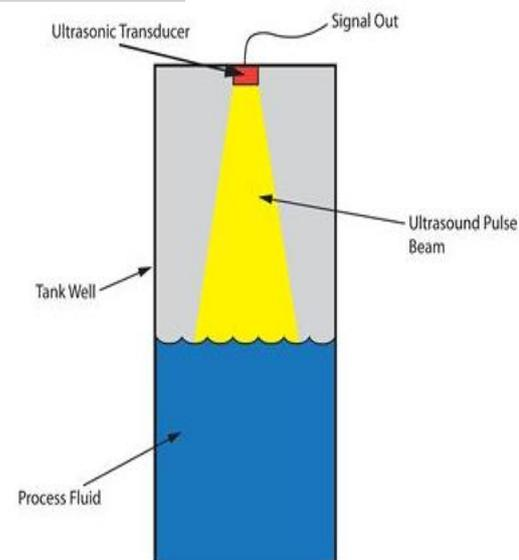
The operational frequency of these transmitters is tens of kilohertz and the transit times are approximately 6 ms/m. The composition of the gas mixture in the headspace and its temperature affect the speed of sound (340 m/s in air at 15°C). Even though the sensor compensates for temperature, it is limited to atmospheric measurements in nitrogen or air.
