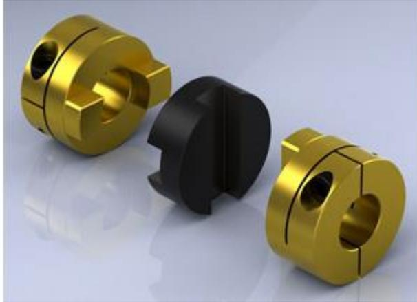
Oldham couplings can accommodate lateral shaft misalignments up to 10% of nominal shaft diameters and up to 3 angular misalignments.
