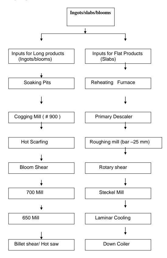
Special steels including Alloy and Stainless have both continuous cast and Ingot teeming products. Grades having high carbon and high alloy are hot transferred. All ingots and continuous cast slab or blooms are charged into soaking pit furnaces.
