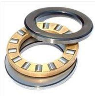
Roller thrust bearings like the one illustrated can support very large thrust loads. They are often found in gear sets like car transmissions between gear sprockets, and between the housing and the rotating shafts. The helical gears used in most transmissions have angled teeth, this can causes a high thrust load that must be supported by this type of bearing. Roller thrust bearing designated as 8XXX
