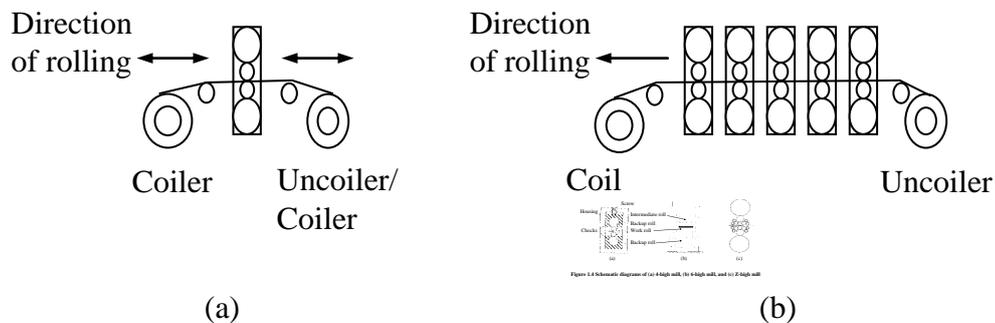
**Schematic of (a) Reversing Mill and (b) Tandem Mill**
