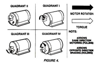
direction and it functions as a conventional non-regenerative unit. The unique characteristics of a regenerative drive are apparent only in Quadrants II and IV. In these quadrants, the motor torque opposes the direction of motor rotation which provides a controlled braking or retarding force. A high performance regenerative drive, is able to switch rapidly from motoring to braking modes while simultaneously controlling the direction of motor rotation.
