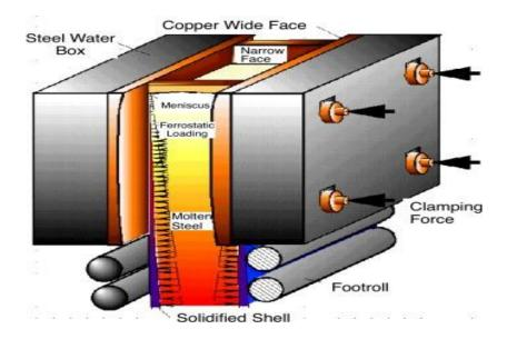
The mould is basically an open-ended box structure, containing a water-cooled inner lining fabricated from a high purity copper alloy. Mould water transfers heat from the solidifying shell. The working surface of the copper face is often plated with chromium or nickel to provide a harder working surface, and to avoid copper pickup on the surface of the cast strand.
