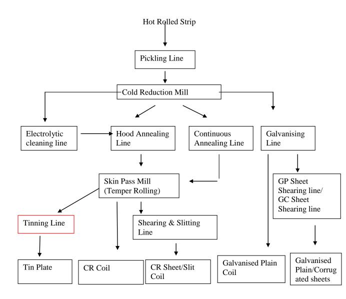
(Fig.3.1: Typical material flow in a Cold Rolling Mill Complex)
