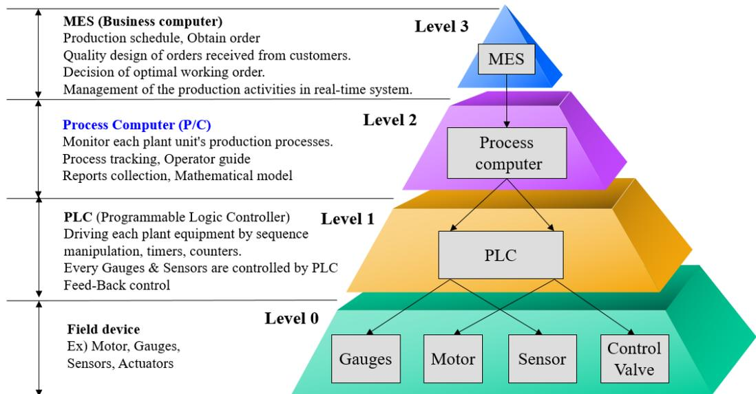
**Level-2 automation** is used for complex processes to optimize the process based on software modelling. The level-2 system also generates plans and schedules for the production and process. Level-2 system takes all the inputs from level-1 system and generates output and set points for the operator as well as for level-1 system.
