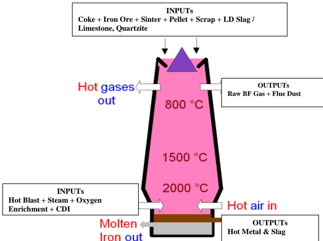
The entire furnace is lined with suitable refractory and in addition to refractory lining, there are water coolers, designed to enhance the life of the furnaces. **In a blast furnace, fuel, Iron ore, sinter and flux (limestone) are continuously supplied through the top of the furnace**, either through 'double bell system' or 'bell less system'. In the hearth, there is a tap hole of suitable dimension and length, for the purpose of tapping the hot metal.
