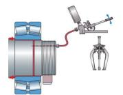
This method can't be used unless provided for in the design of mounting. Special oil injection tool is required. After mounting of bearings the axial float of the bearing should be as per OEM recommendation.
