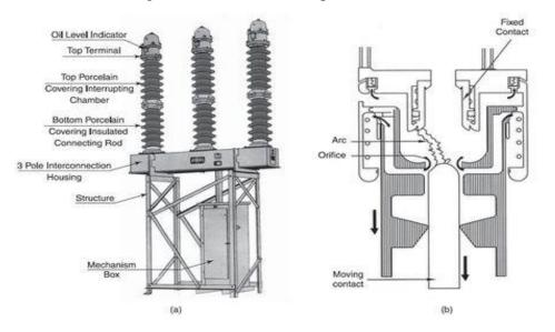
36 kV MOCB a) Typical design, b) Cross-section of the interrupting chamber
