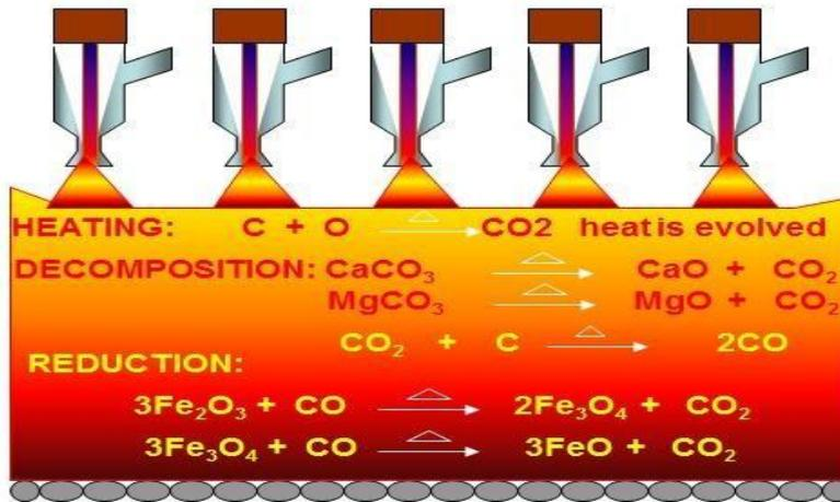
The gases used in ignition furnace are mainly coke oven gas or mixed gas. Mixed gas is combination of coke oven gas and blast furnace gas. Further the combustion is continued due to suction of air through the layers of the charge by means of Exhausters. Due to this, the process of combustion of fuel gradually moves downwards up to the grates.
