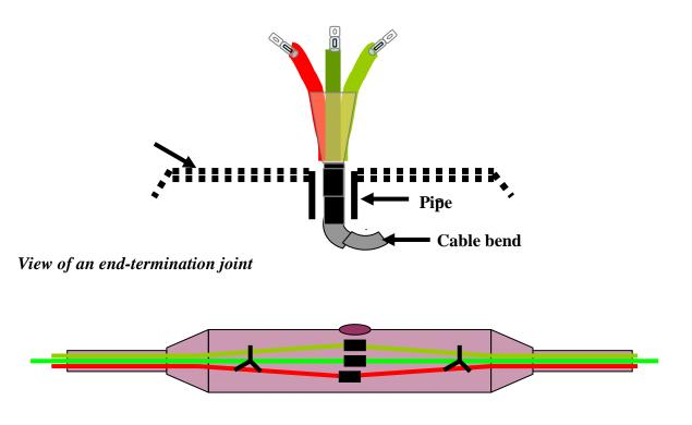
Cross-sectional view of a Straight-through Joint
