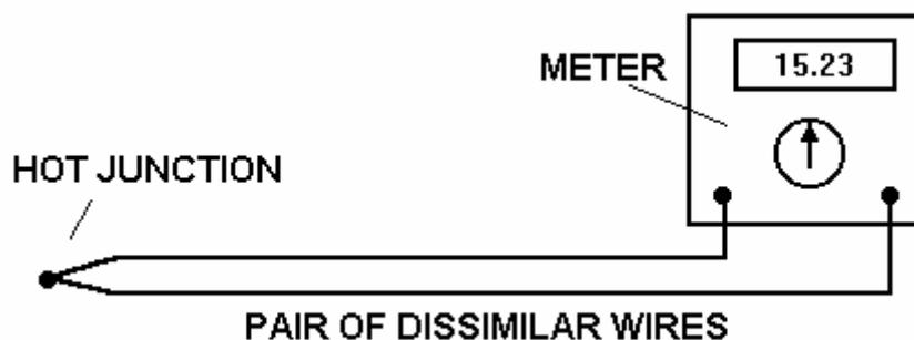
Most thermocouple metals produce a relationship between the two temperatures and the e.m.f as follows.
