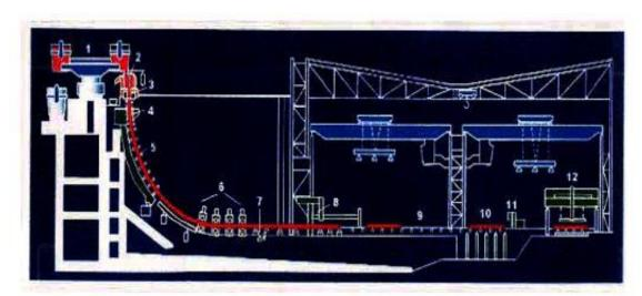
Figure 2 - General Bloom/Beam Blank Machine Configuration
