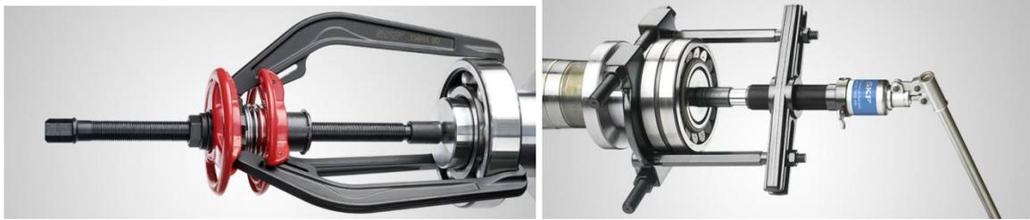
For dismounting of plain bore bearings mechanical/hydraulic bearing pullers & press should be used. Direct hammering should be avoided as it may damage the bearing.
