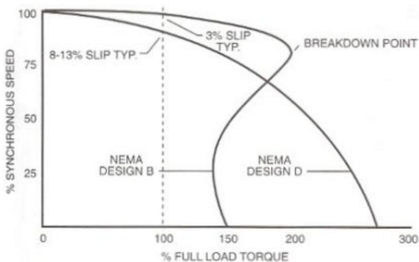
**FIGURE 9. Typical Speed-Torque Characteristics at Rated Voltage & Frequency**
