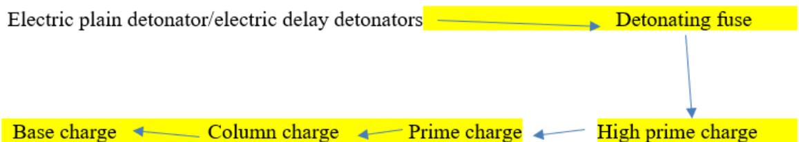
Delay sequencing is managed between the rows by use of the electric delay detonators which are connected in series and fired by an exploder.
