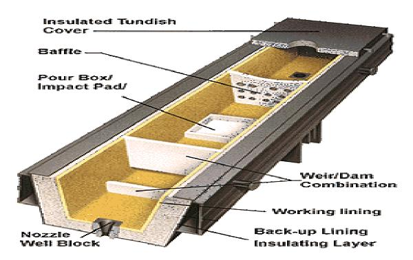
The shape of the tundish is typically rectangular, but delta and "T" shapes are also common. Nozzles are located along its bottom to distribute liquid steel to the moulds. The tundish also serves several other key functions:
