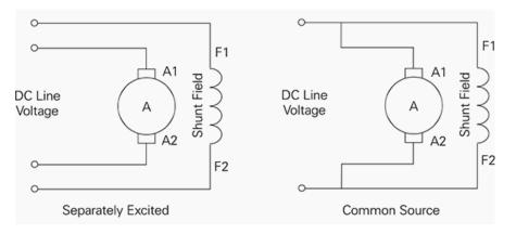
In a shunt motor the field is connected in parallel (shunt) with the armature windings. The shunt-connected motor offers good speed regulation. The field winding can be separately excited or connected to the same source as the armature
