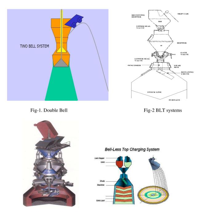
Fig-3 Rotary Charging Unit (RCU) Fig-4 BLTCharging
