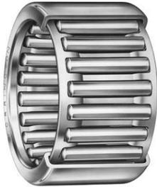
A variation of roller bearing design is called the needle bearing. The needle roller bearing uses cylindrical rollers like those above but with a very small diameter. This allows the bearing to fit into tight places such as gear boxes, cardan shafts that rotate at higher speeds & also has a more load carrying capacity.
