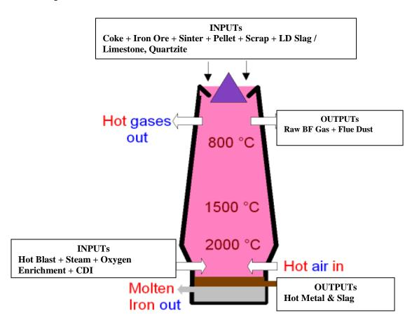
The entire furnace is lined with suitable refractory and in addition to refractory lining, there are water coolers, designed to enhance the life of the furnaces. In a blast furnace, fuel, Iron ore, sinter and flux (limestone) are continuously supplied through the top of the furnace, either through 'double bell system' or 'bell less system'. In the hearth, there is a tap hole of suitable dimension and length, for the purpose of tapping the hot metal.
