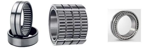
Cylindrical roller bearings generally are single row bearings with a cage. High-capacity bearings, double row bearings, multi-row bearings, single, double and multi-row full complement bearings (without a cage) and split bearings are other varieties. Bearings with a cage can accommodate heavy radial loads, rapid accelerations and high speeds. Full
