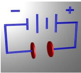
A parallel plate capacitor is shown in the adjoining figure, connected to a battery. The potential difference across the plates of the capacitor is equal to the battery voltage, thereby charging the capacitor. However due to the inherent nature of
