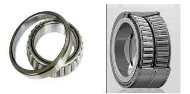
Tapered roller bearings are designed to support large radial and large thrust loads. These loads can take the form of constant loads or shock loads. Tapered roller bearings are used in many gear boxes, where they are usually mounted in pairs facing opposite directions. This gives them the ability to take thrust loads in both directions. Taper roller designated as 3XXX in metric size & in inch size 9XX/9XX.
