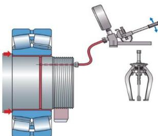
This method can't be used unless provided for in the design of mounting. Special oil injection tool is required.
