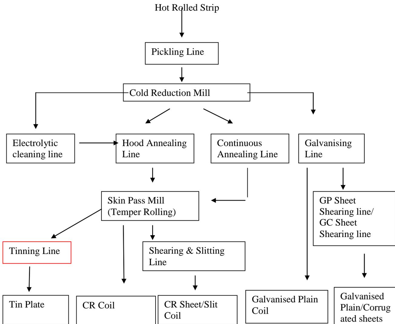
(Fig.3.1: Typical material flow in a Cold Rolling Mill Complex)
