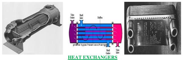
In shell and tube type heat exchangers the cooling fluid flows in the bunch of tubes placed inside the shell while the fluid to be cooled flows, in a reverse direction, in the shell, in the leftover gaps between the tubes.
