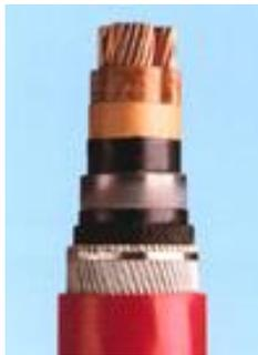
**PILC cables** are widely used for LV and MV applications. Insulation between the conductors and overall insulation over the cable is provided by liquid-impregnated electrical grade paper. A lead sheath over the paper insulation provides mechanical protection for the insulation, encapsulating the impregnated fluid, and prevents environmental degradation. The lead sheath also provides a ground path under fault conditions.
