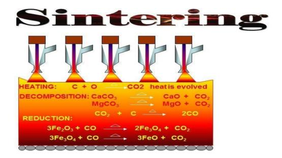
The gases used in ignition furnace are mainly coke oven gas or mixed gas. Mixedgas is combination of coke oven gas and blast furnace gas. Further the combustion is continued due to suction of air through the layers of the charge by means of Exhausters. Due to this, the process of combustion of fuel gradually moves downwards up to the grates.
