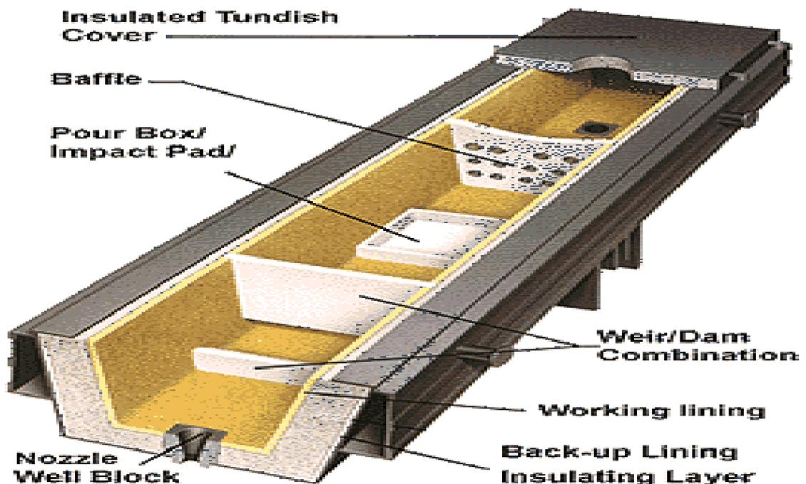
The shape of the tundish is typically rectangular, but delta and "T" shapes are also common. Nozzles are located along its bottom to distribute liquid steel to the moulds. The tundish also serves several other key functions:
