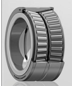
Tapered roller bearings are designed to support large radial and large thrust loads. These loads can take the form of constant loads or shock loads. Tapered roller bearings are used in many gear boxes, where they are usually mounted in pairs facing opposite directions. This gives them the ability to take thrust loads in both directions. Taper roller designated as 3XXX in metric size & in inch size 9XX/9XX.
