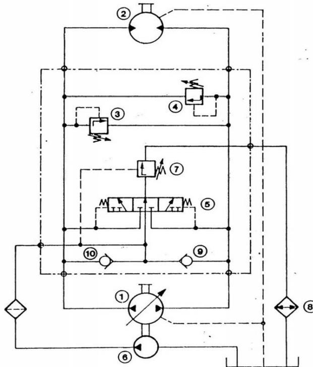
In the closed hydraulic the oil after rotating the hydro motor doesn't go to the tank back, instead it goes to the pump's suction line again. In this process the same oil is only circulating. To take care of the mixing of cool and fresh oil from the tank a booster pump is installed which is normally in tandem with the main pump. It mixes the oil from the tank to the circuit through a flushing valve.
