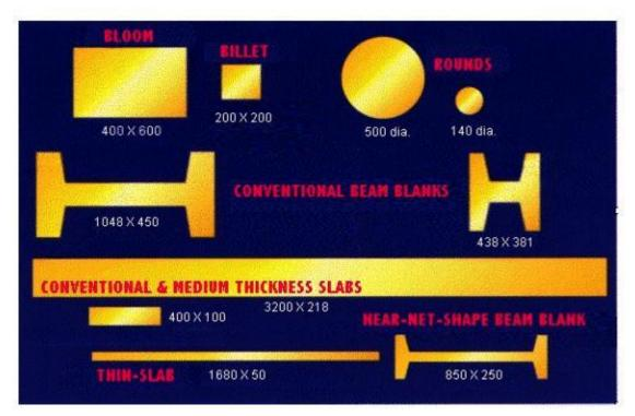
Figure 4 - Continuous Cast Shapes (sizes in millimeters)
