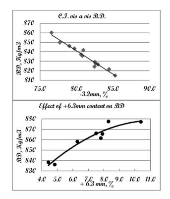
Fig : Bulk density variation with Crushing Index and +6.3 mm content in coal charge
