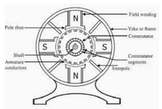
The outer frame of the motor is called yoke that serves two purposes.
