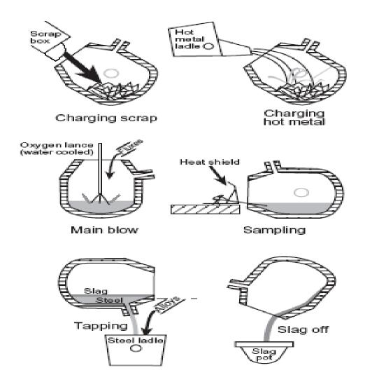
Basic Oxygen Furnace is commonly known as BOF process or LD process. It is named so because this process was developed in LINZ and DONAWITZ, two cities in Austria. The process is also called basic because of refractory type used for lining the vessel to withstand the high temperature of molten metal.
