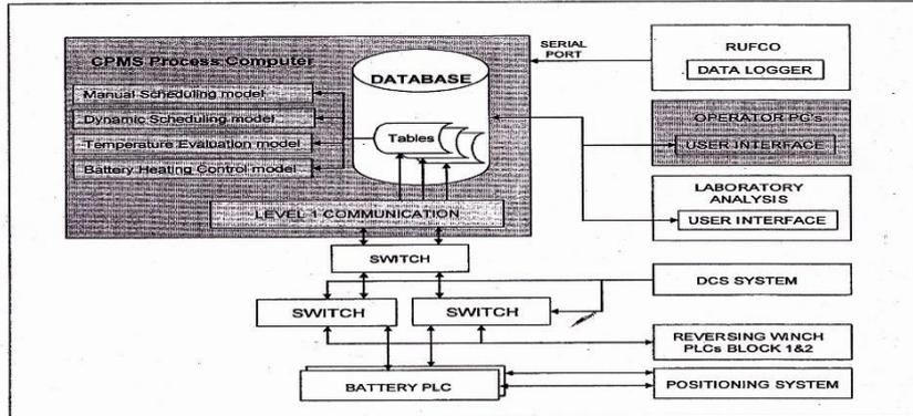
Figure 1 CPMS logical structure and main data flows
