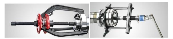
For dismounting of plain bore bearings mechanical/hydraulic bearing pullers & press should be used. Direct hammering should be avoided as it may damage the bearing.
