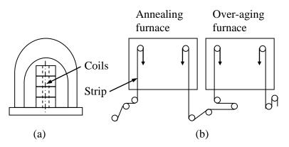
Figure: Schematics of (a) Batch Annealing and (b) Continuous Annealing
