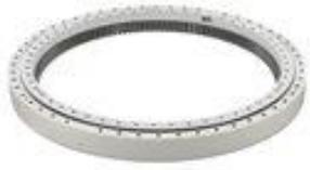
This bearing can take radial, axial & tilting loads. Slewing bearings are generally manufactured in very large diameters & fixed by bolting. These are found application in blast furnace clay gun & tap hole drill machine, Caster ladle turret & heavy cranes. Plain & gear (internal & external) are two varieties.
