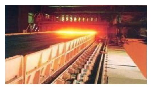
Fig1: Sinter Machine at SP3, Machine 1
