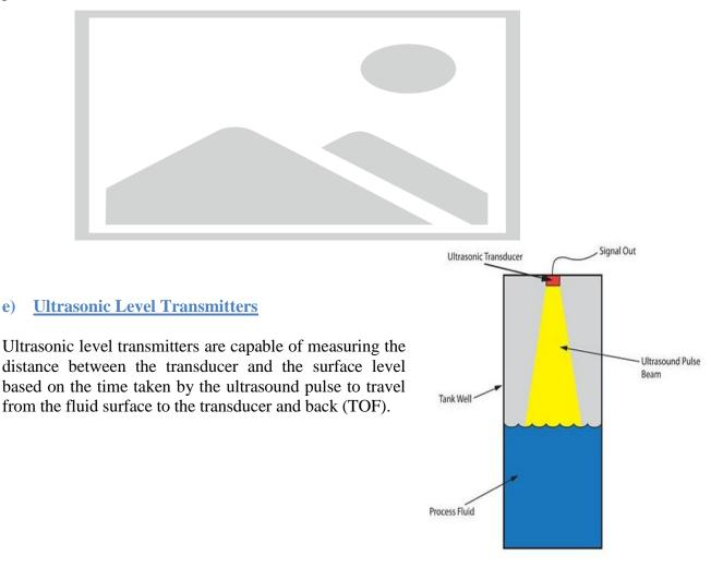
The operational frequency of these transmitters is tens of kilohertz and the transit times are approximately 6 ms/m. The composition of the gas mixture in the headspace and its temperature affect the speed of sound (340 m/s in air at 15°C). Even though the sensor compensates for temperature, it is limited to atmospheric measurements in nitrogen or air.
