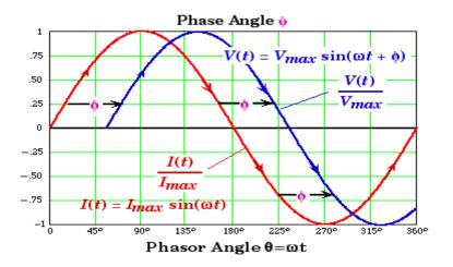
The angle by which the sine curve of the voltage in a circuit leads or lags the sine curve of the current in that circuit is called the phase angle  $\emptyset$ . If  $\emptyset$  is positive the voltage leads the current.
