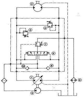
In the closed hydraulic the oil after rotating the hydro motor doesn't go to the tank back,
