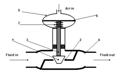
Fig.1 Air-to-close pneumatic actuator with valve
