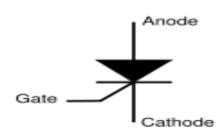
unidirectional conduction. The term **Thyristor is often** used in literature as a synonym of the SCR.
