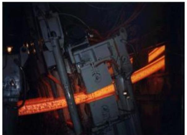
After straightening, the strand is transferred on roller tables to a cut off machine, which cuts the product into ordered lengths. Sectioning can be achieved either via torches or mechanical shears. Then, depending on the shape or grade, the cast section will either be placed in intermediate storage, hot-charged for finished rolling or sold as a semi-finished product.
