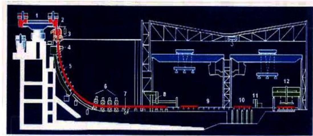
*1:Ladle Turret, 2:Tundish/Tundish Car, 3:Mould, 4:First Zone (Secondary Cooling), 5:Strand Guide (plus Secondary Cooling), 6:Straightener Withdrawal Units, 7:Dummy Bar Disconnect Roll, 8:Torch Cut-Off Unit, 9:Dummy Bar Storage Area, 10:Cross Transfer Table, 11:Product Identification System, 12:Product Discharge System*
