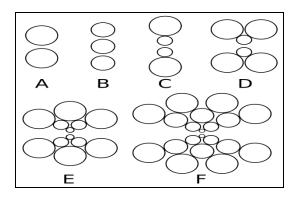
Various rolling configurations. Key: A. 2-high B. 3-high C. 4-high D. 6-high E. 12high cluster & F. 20-high <u>Sendzimir Mill</u> cluster
