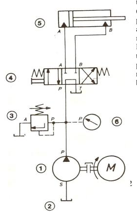
the pump flow and the cylinder size (piston area). The force available at the piston rod is dependent on the piston area and the maximum system pressure. The maximum system pressure and thus the loading of the hydraulic system is set at the pressure relief valve 3. The actual pressure available, determined by the resistance to be overcome at the user, can be read at the pressure gauge 6.
