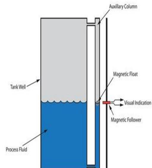
The float is laterally confined by the column so it remains close to the side wall of the chamber. The position of the float moves up and down according to the fluid level, which is indicated by a magnetized shuttle or a bar graph that moves along with it, showing the float's position and thereby indicating the level.
