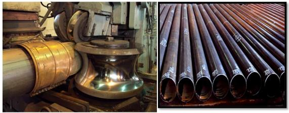
Hot rolled coils (from Hot Strip Mill of RSP or from out side sources like BSL) are the main input material for ERW Pipe Plant. This input material is cold formed to a tubular shape by gradual deformation and then welded by the combination of heat and pressure.
